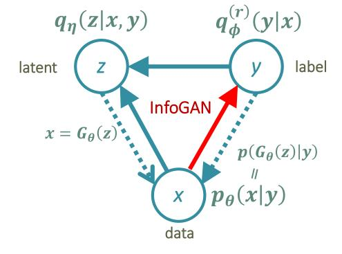
"Schematic graphical model of Adversarial Autoencoder (AAE), which is obtained by swapping data x and code z in InfoGAN."
