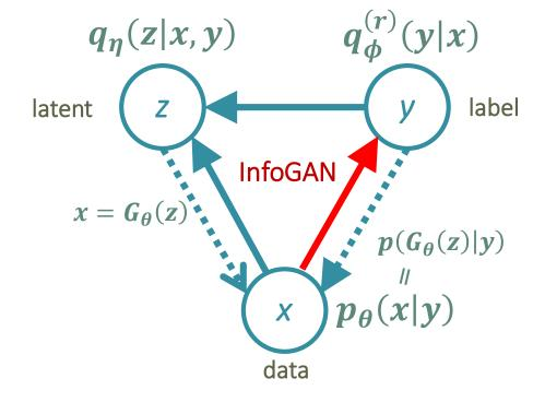
"Schematic graphical model of VAEs, which is obtained by **swapping the generative and inference processes** of InfoGAN."
